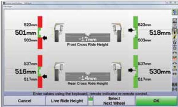
*Color-coded bar graphs show adjustments needed to set ride height within the vehicle's specifications.*
