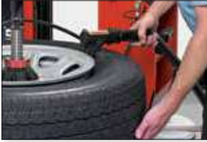
Blast inflation directs large blast of air for tough bead seating.
