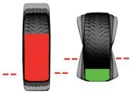
SmartWeight<sup>®</sup> panel displays wheel balance condition
