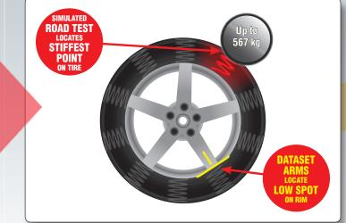
The Road Force Touch balancer detects radial forces with sensitive instruments
