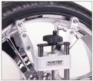
Optional extensions snap into place providing a safe, rigid clamp for wheels up to 28 inches in diameter.
