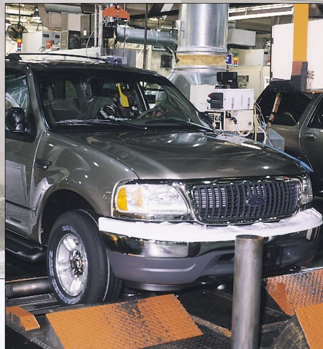
High-volume test lines audit the newly assembled vehicles for excessive vibration at highway speeds.
