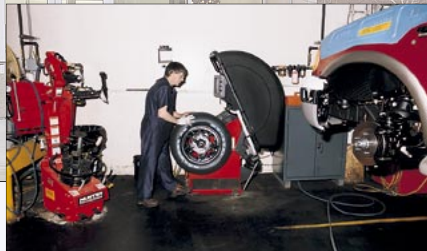
Ford factory technicians diagnose and correct out of specification tire and rim assemblies using Hunter's GSP9700 Vibration Control System and TC3500 Euro-style tire changer.
