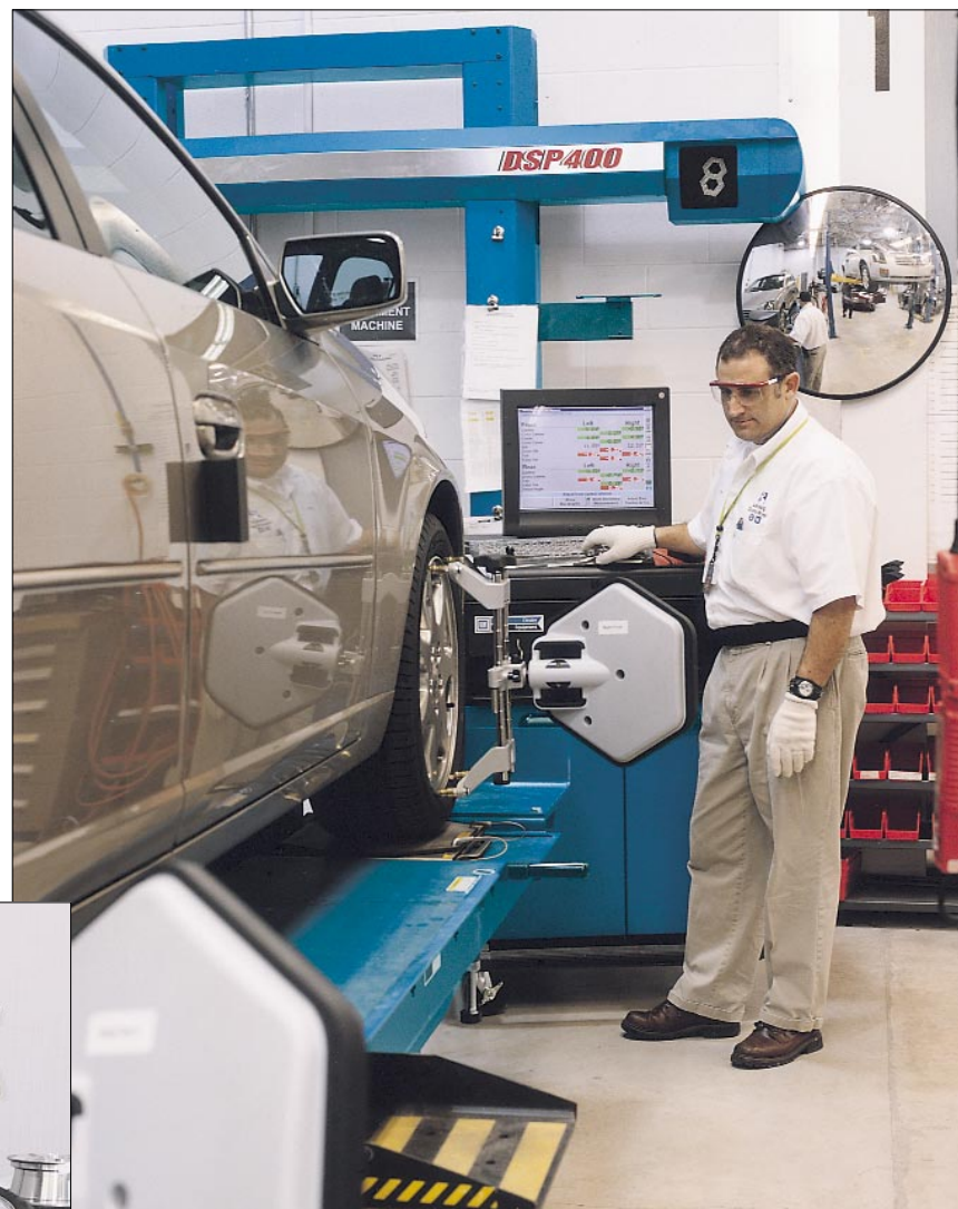
Cadillac Quality Assurance Director Tom Rizzo (above) uses an off-the-shelf Hunter-GM 611 with DSP400 sensors to get alignment measurements on this early production model CTS.
