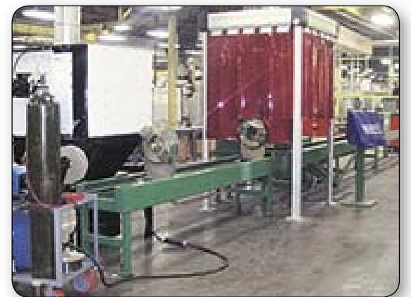
The MasterTube Plasma Cutter begins production of RX lifts by transforming 20-foot pieces of steel tubing into scissor legs.
