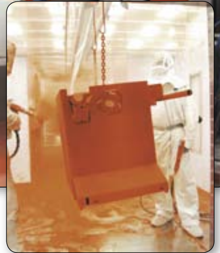
The multi-stage powder coat line cleans, coats and cures parts for final assembly (above). Though most of the application is automated, Raymond staff ensure quality by evening out the finish when necessary (right).
