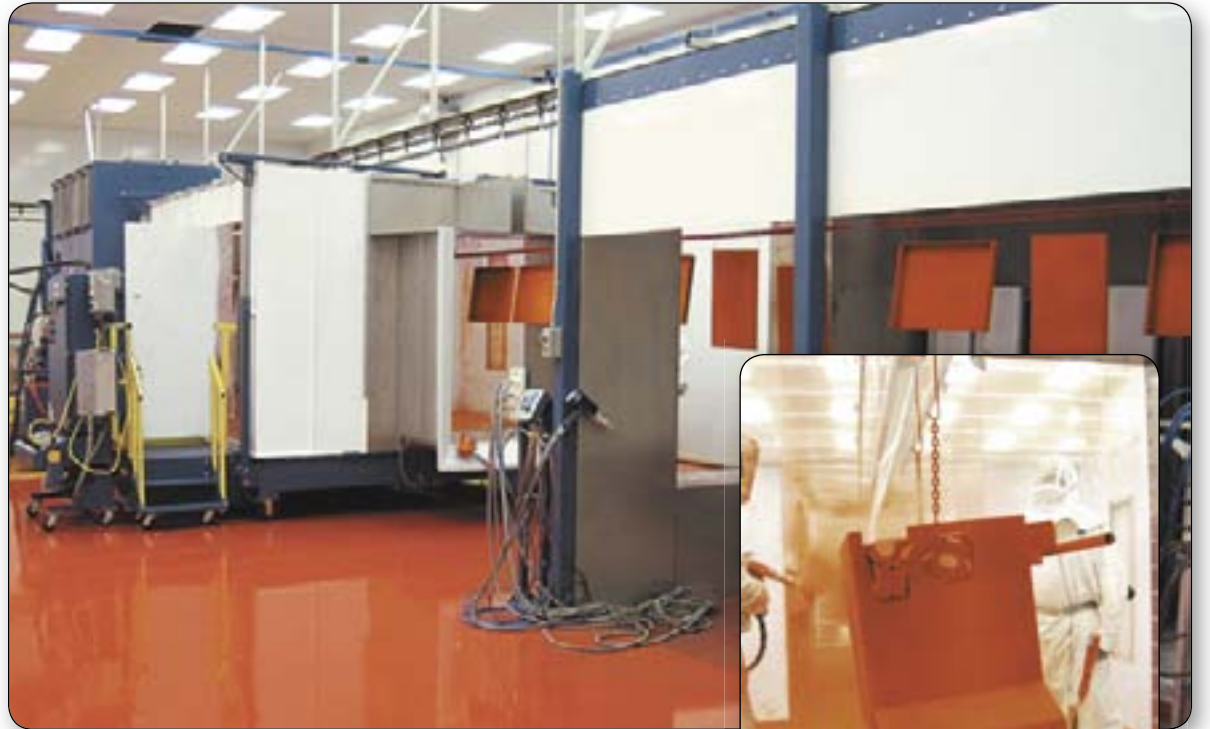
The multi-stage powder coat line cleans, coats and cures parts for final assembly (above). Though most of the application is automated, Raymond staff ensure quality by evening out the finish when necessary (right).
