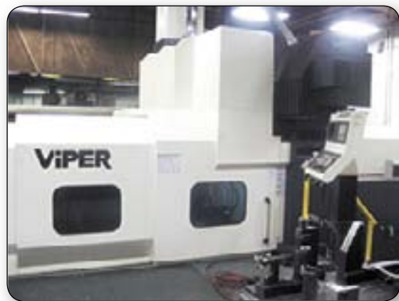
The Viper provides precise milling and drilling of many other Hunter product parts along with the RX lift legs.
