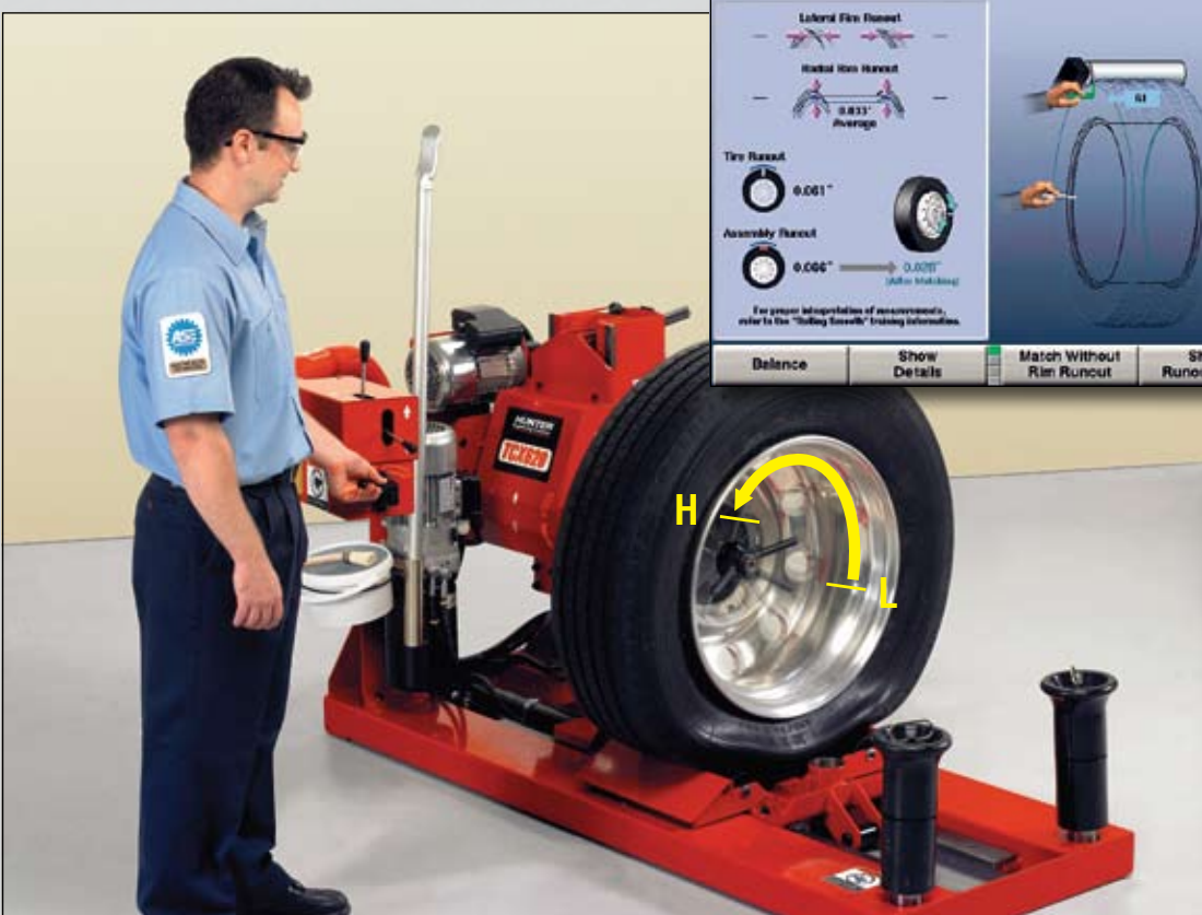
By following simple on-screen instructions, a technician can minimize vibration through match-mounting the high spot on a tire to the low spot on a rim.
