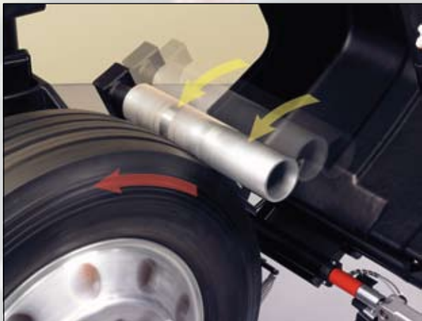
The loaded roller contacts the entire footprint of the tire, providing a 360° evaluation.
