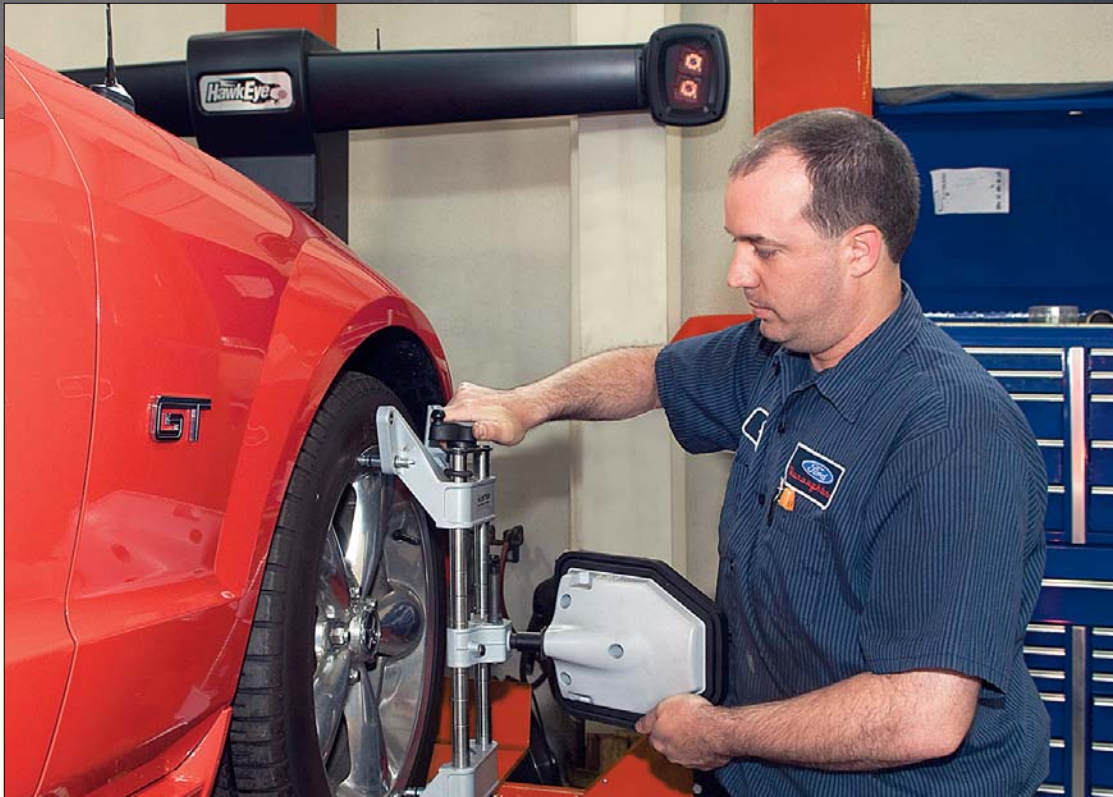
At Thoroughbred Ford in Kansas City, technician Tim Heimberger sets up his next job using a new Hunter HawkEye™ high-definition alignment system from Rotunda.
