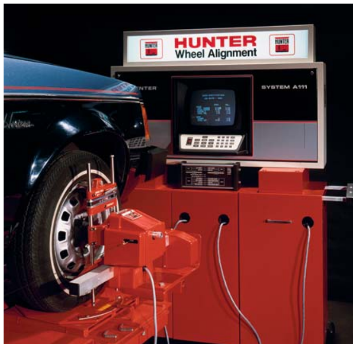
This Hunter A111-D4M model aligner featured a mobile cabinet with self-illuminated signage. Four-wheel electronic sensors were hard-wired to the cabinet.
