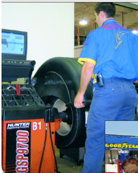
Assemblies are then remeasured for excessive vibration and balanced using eight GSP9700s.
