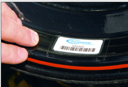
Champion archives and tracks data on every wheel throughout its life. The data is quickly accessed using a bar code scanner.
