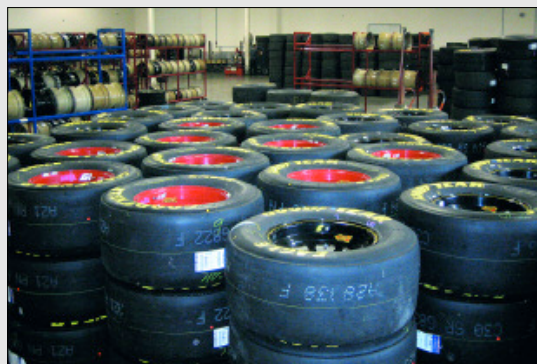
Daily output can reach 1200 match-mounted tire and wheel assemblies, or more than 100,000 per season. These wheel assemblies will be used for testing. Wheels used in races are assembled at the track on the day of the event.
