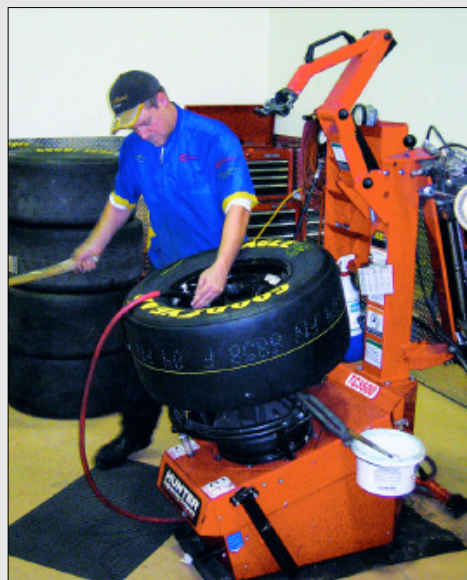
Champion technicians use Hunter TC3500 Tire Changers to match-mount all tire and wheel assemblies prepared at their North Carolina facility.
