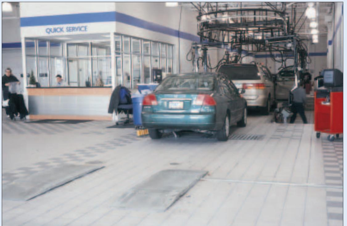
*Vehicles entering the automated maintenance lane are first tested for excessive sideslip. The SS100 measures each axle and shows results instantly on the console screen.*
