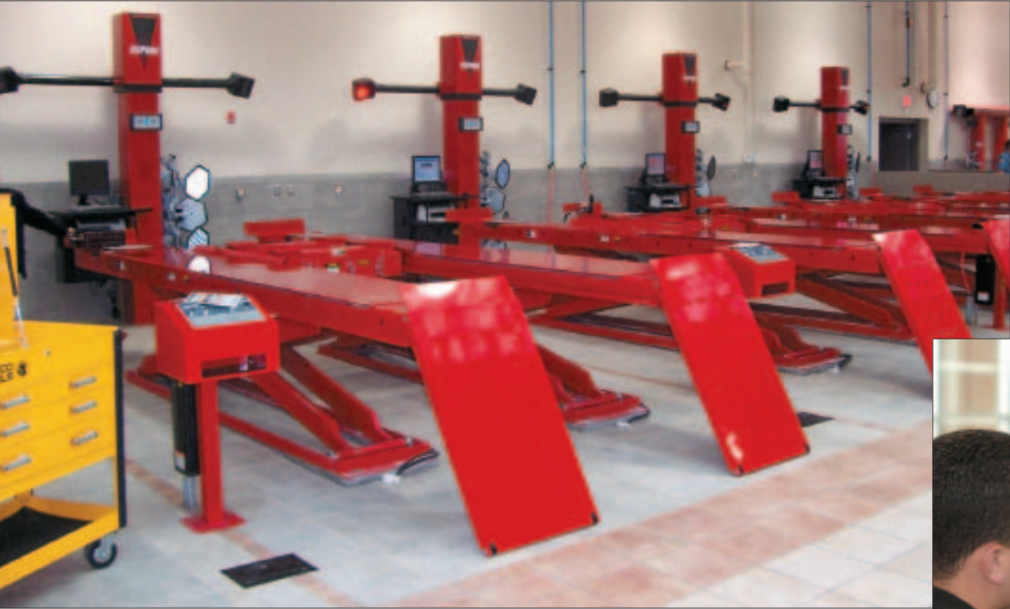
These newly installed alignment bay classrooms use Hunter W811P-Plus cabinet configurations matched with DSP600 digital imaging alignment sensors and RX alignment racks. The school also provides alignment instruction using conventional electronic sensors to provide students with experience using the widest range of equipment types that they may encounter in the workplace.
