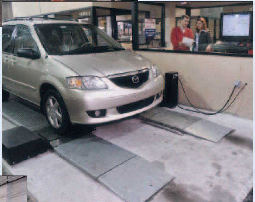
The write-up areas are climate-controlled booths. The lanes provide a complete Hunter automated undercar inspection including an actual brake performance test, suspension analysis and wheel sideslip reading.
