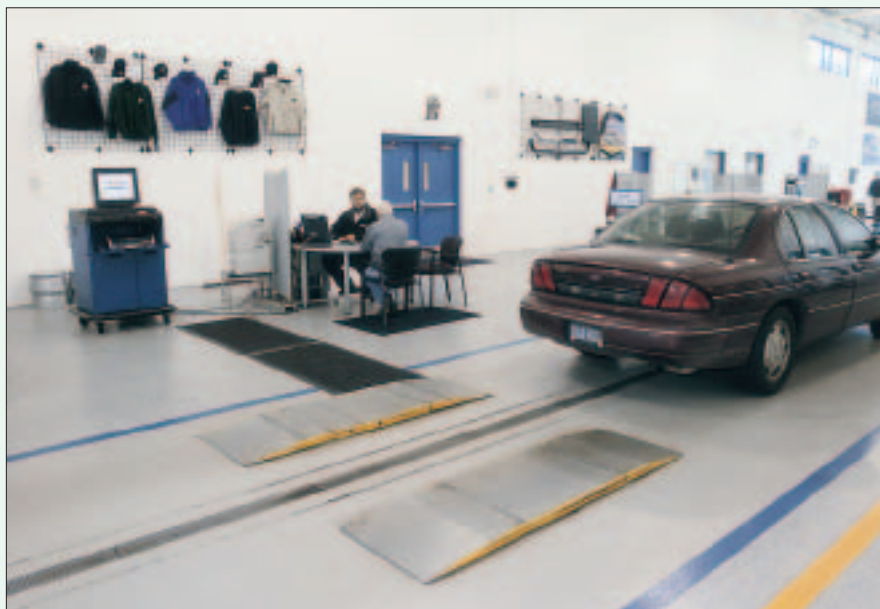
All vehicles arriving at Young Chevrolet–Oldsmobile–Cadillac travel over SS100 sideslip plates. A printout is provided immediately by the system console.
