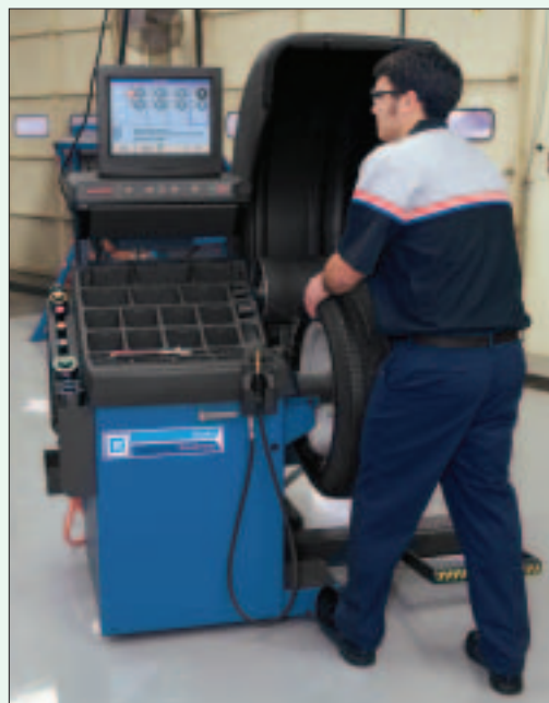
Young's service department uses a Hunter GSP9700 Road Force Measurement® system like the unit shown above. After performing a computerized road test, the GSP9700 calculates the rim and tire's contribution to excessive radial vibration and shows the technician step-by-step repair instructions.
