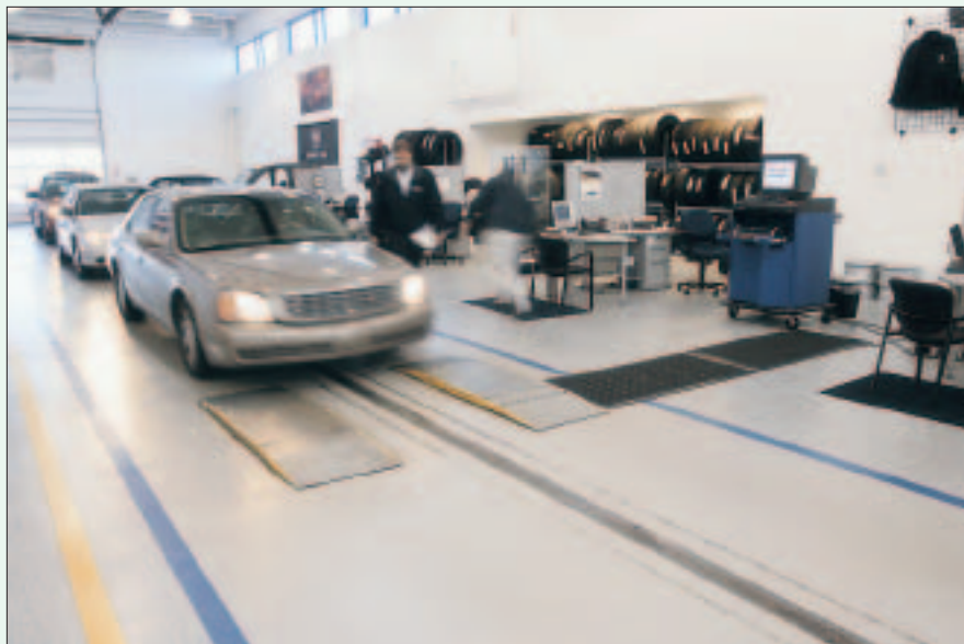
All vehicles arriving at Young Chevrolet–Oldsmobile–Cadillac travel over SS100 sideslip plates. A printout is provided immediately by the system console.
