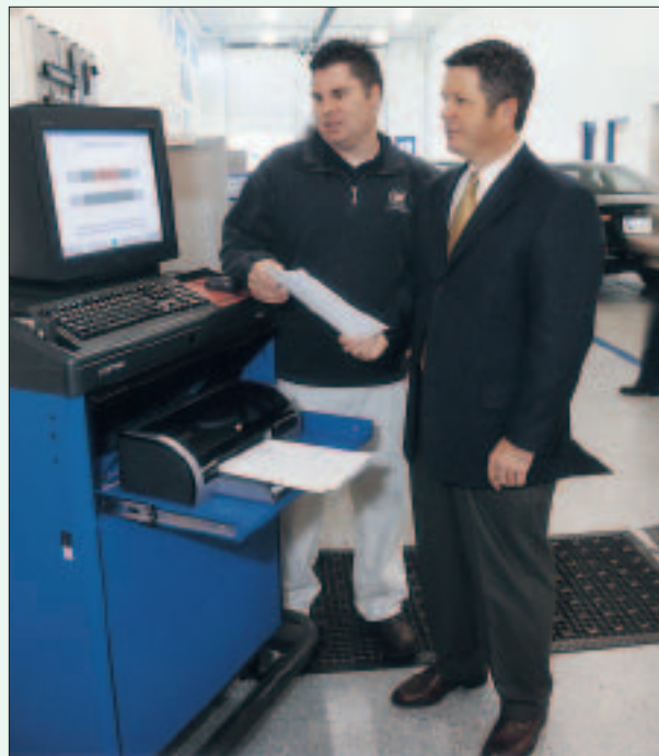
Young Chevrolet–Oldsmobile–Cadillac owner Tony Young and lead service writer Joe “J.T.” Thibault examine printed sideslip meter test results that may indicate vehicle misalignment or damaged or worn parts.
