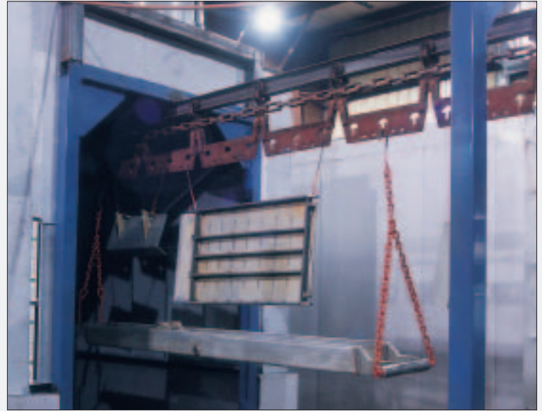
In a highly automated process parts receive a phosphate wash and are dried in ovens prior to application of the resin powder.
