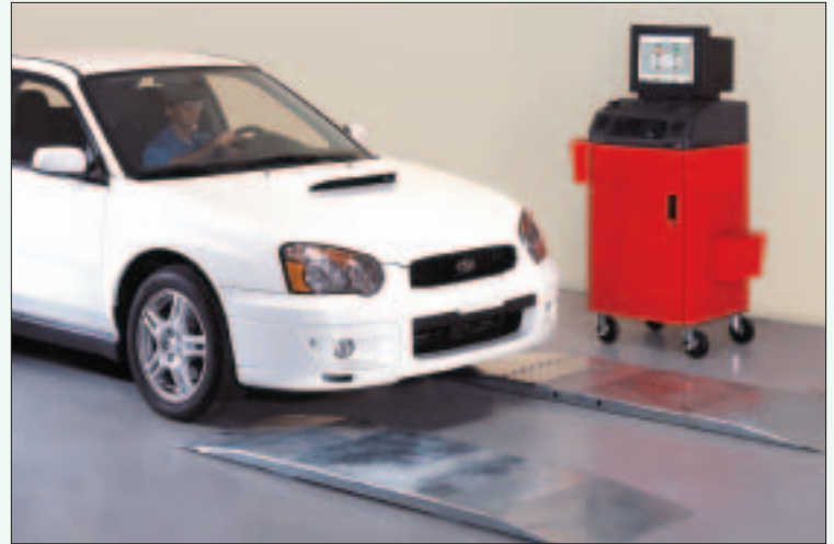
Above, the SS100 displays vehicle sideslip on the Windows-based computer console screen. Left, the SS100T handles heavy-duty trucks as well as passenger cars.
