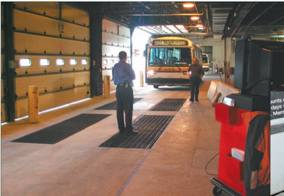
One of three Hunter B400T brake testing lanes at NFTA maintenance facilities in the Buffalo/Niagara Falls metropolitan area.
