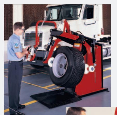
unter has added an innovative new product to its heavy-duty truck service equipment line. The TC2450HD Heavy-Duty Tire Changer is an advanced design with patented features that make mounting and demounting truck tires quick and easy. The machine does the hard work, placing fewer stresses on the tire and rim, and the operator. A high production shop can keep one technician changing tires all day without the fatigue associated with traditional methods.
