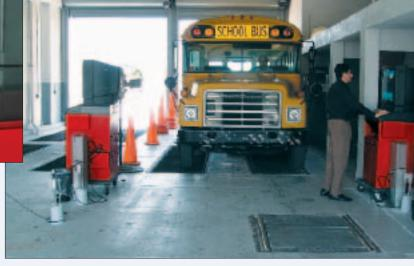
Each lane is also equipped with a Hunter SS100T Sideslip meter (floor-mounted plate is visible at bottom of photo).
