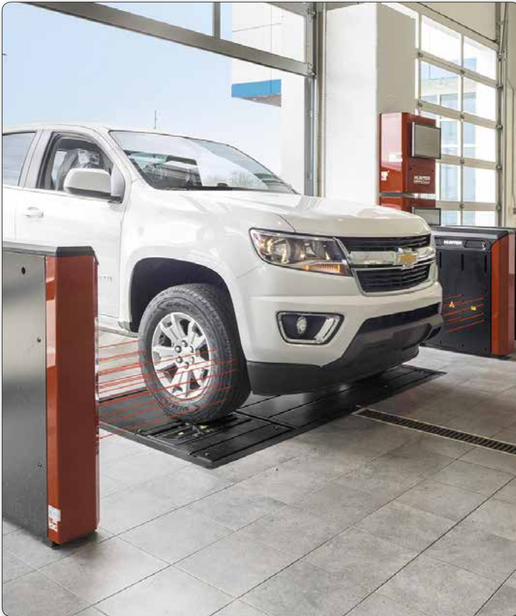
Hunter's touchless alignment inspection system uses laser technology to measure camber and total toe in seconds.
