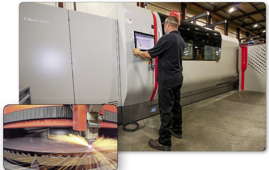
Above: The cut head is positioned by three linear induction motors capable of 2g acceleration, the equivalent of 0-60 in 1.37 seconds.
