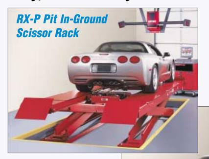
unter's RX-P Scissor Lift Rack is an above-ground lift installed in a shallow pit, providing flush-to-the-ground runways for entry and exit. This feature all but eliminates clearance worries when servicing low-to-the-ground vehicles. The RX-P drive-through configuration (shown with DSP600WMS Sensors) provides even greater compatibility with low spoiler- or air damequipped vehicles. The RX-P is a clean, efficient,
