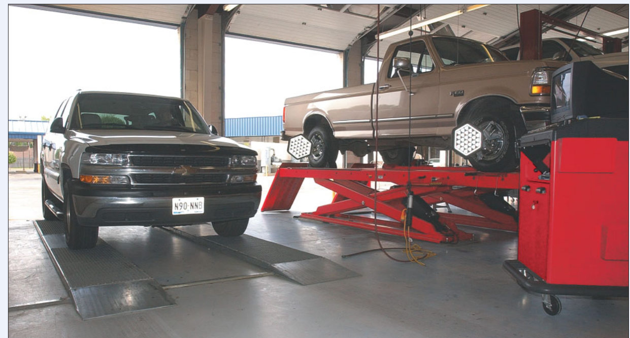
Pictured at left, a vehicle is driven from the lube center through the Inspection lane for a brake performance test and sideslip inspection that takes less than sixty seconds. A color printout of test results, pictured below, helps All American staff explain needed service. The All American Super Wash & Lube Center is pictured at bottom.
