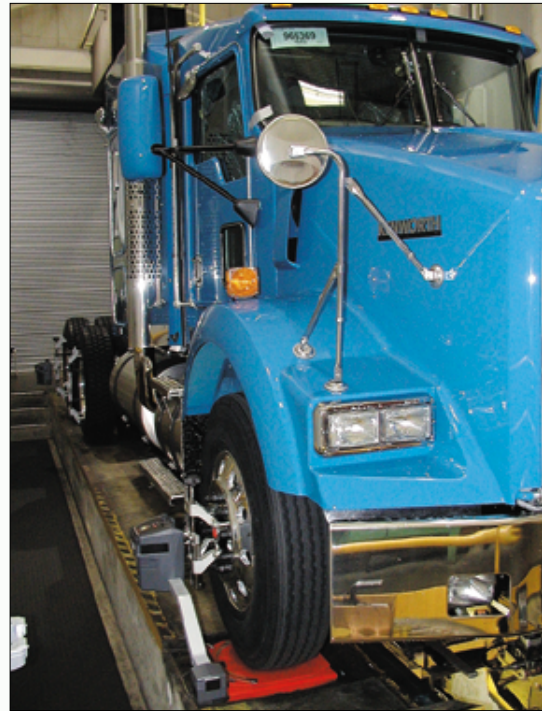
Kenworth technicians align newly-built Class 8 trucks using Hunter 611T heavy-duty alignment systems and DSP306 cordless sensors.
