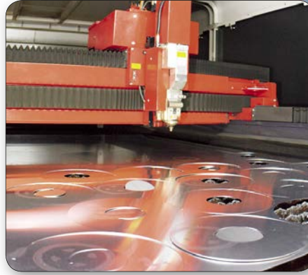
A laser cutter in Hunter's Raymond plant cuts aluminum for Road Force balancer load rollers.
