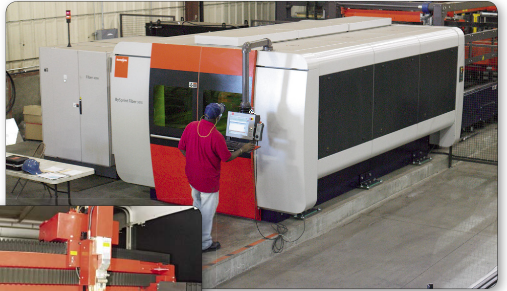
A laser cutter in Hunter's Raymond plant cuts aluminum for Road Force balancer load rollers.
