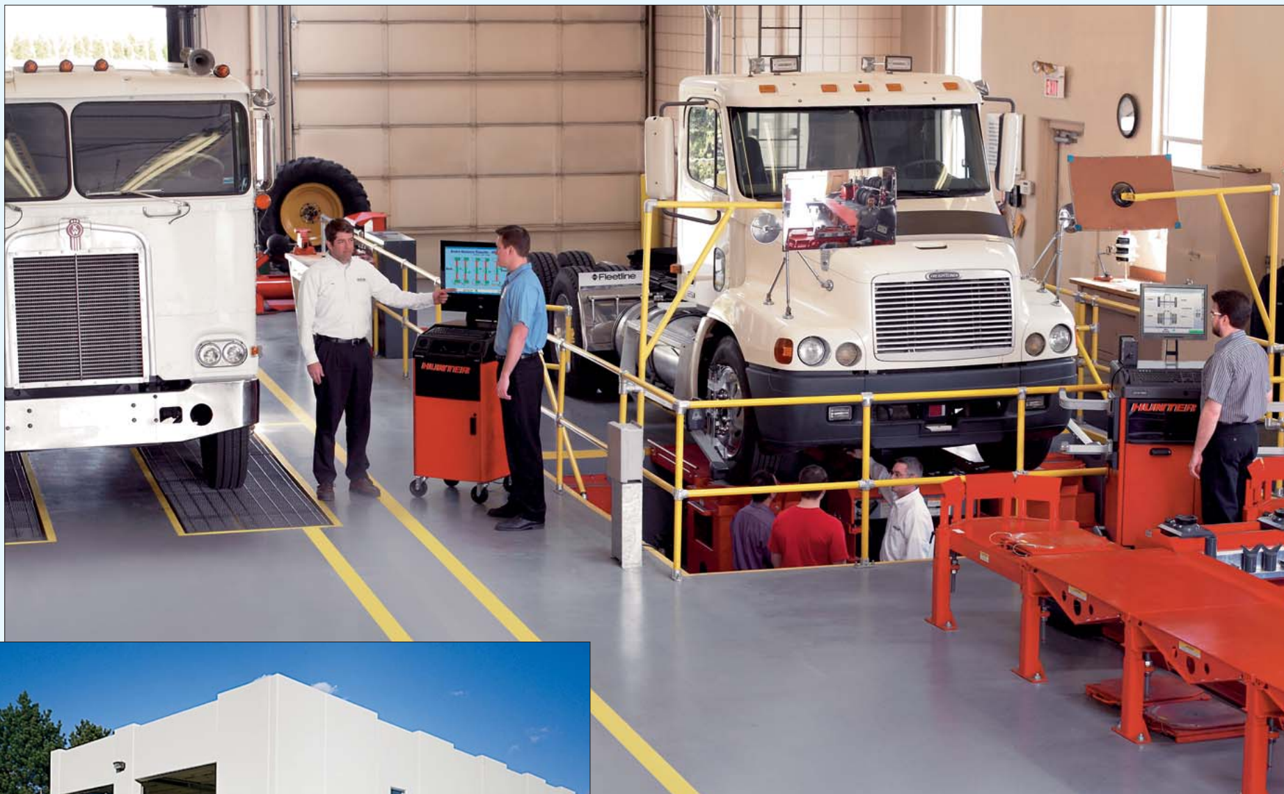
Hunter's Heavy-Duty Truck and Bus Safety Center, part of the St. Louis Research and Training Center complex, has two service lanes with pit racks and a full-length brake and alignment testing lane for tractors and trailers.
