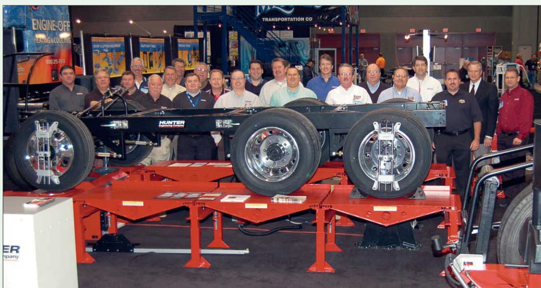
Hunter Heavy-Duty Sales Representatives used a special truck chassis fabricated by company engineers to demonstrate actual truck and trailer alignment procedures. The chassis is elevated on a Hunter RKHD Heavy-Duty Power Rack.
