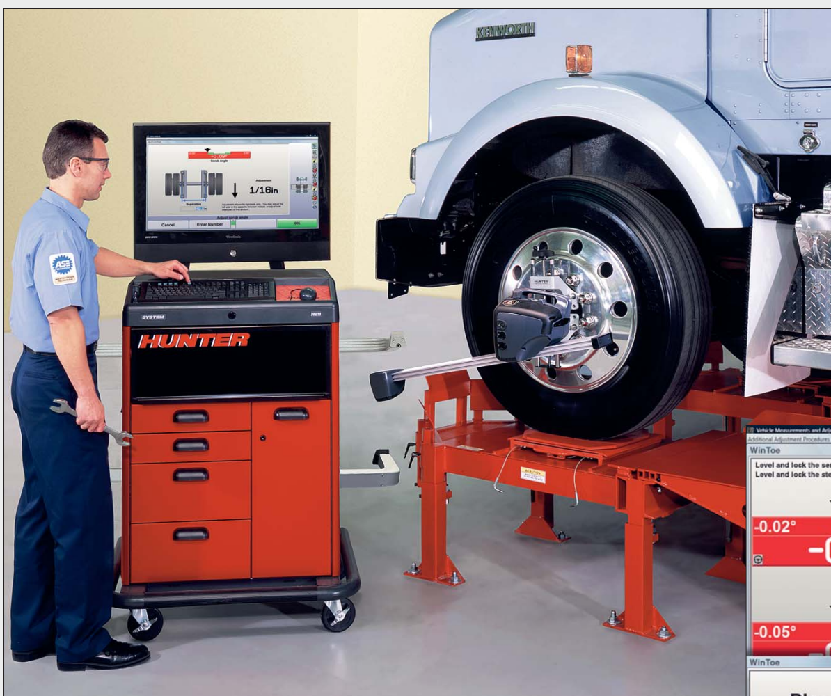
Pictured at right, Hunter's WinAlign®HD alignment software includes the patented WinToe® feature, the quickest and easiest way to align Freightliner's new rack and pinion steering without having to re-center the steering wheel.
