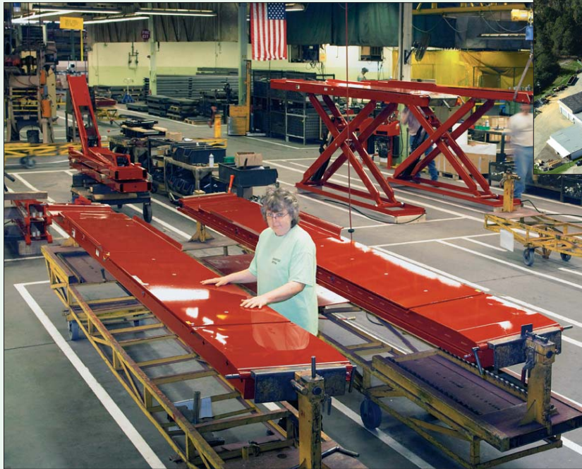
Pictured at left, freshly powder coated RX alignment rack runways are prepared for final assembly. Below, welders fabricate the larger lift rack components by hand. Robotic welders are also used at the plant when appropriate for high-speed, repetitive processes. At bottom left and right, CNC technology speeds production and allows the fabrication of advanced designs.
