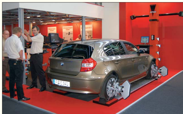
Hunter's leading export product is wheel alignment systems. This Series 811 aligner with DSP600 camera-based sensors took center stage at the exhibit.
