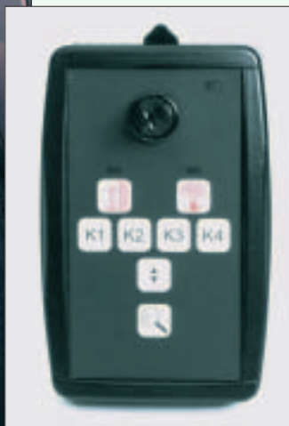
The Hand-Held Ride Height Remote is accurate to within one millimeter.
