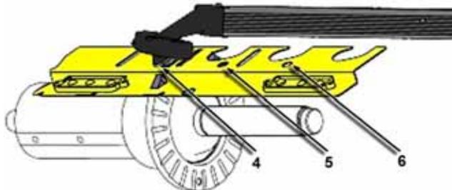
Place the outer Dataset® arm ball in the hole for position “4.” Tap the foot pedal once or press “Enter Cal Step.”
