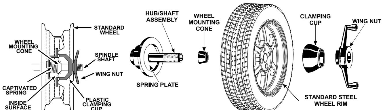
Wheels with center holes over 3 9/16 inch diameter require the light truck cone. The light truck cone can be installed from the outside of the wheel. (When using the light truck cone, the plastic clamping cup is not used.)
