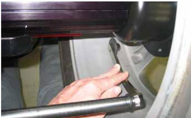
The rim profile can be scanned starting with the rim lip, or from the inside of the wheel. Place the dataset arm against the rim at the desired location, **depress and hold** the foot pedal. The RimScan screen will automatically appear.
