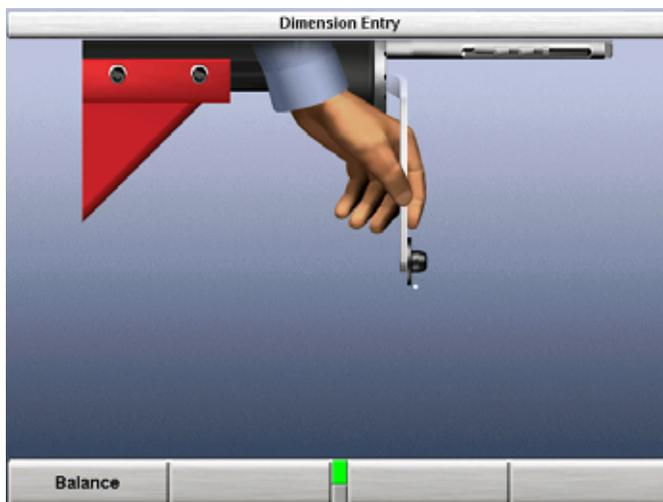
As shown below, draw the dataset arm across the rim to produce an on-screen, live progress of the wheel representation. While it is not necessary to “draw” slowly with the dataset arm, it will produce a more accurate representation of the rim profile especially with rims having multiple steps or taper.
