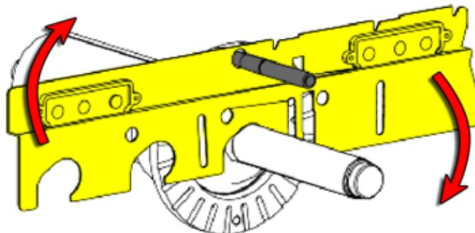
Position the calibration tool parallel to the floor. Tap the foot pedal once or press “OK.”
