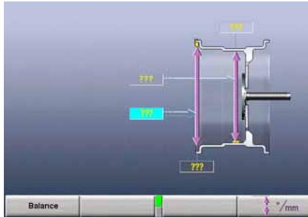
Measure the distance from the left weight plane to the desired right weight plane, using a tape measure. This distance must be in millimeters (convert inches to millimeters by multiplying by 25.4). Measure the weight plane diameter manually, using caliper or tape measure.
