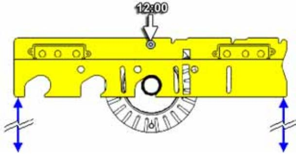
Place the inner Dataset<sup>®</sup> arm at upward position “1.” Tap the foot pedal once or press “Enter Cal Step.”
