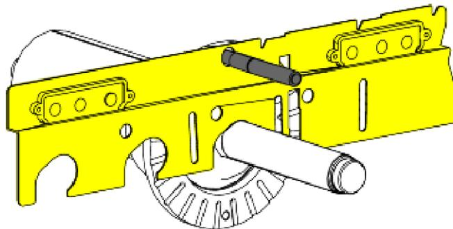
**CAUTION:** Do NOT operate balancer with calibration tool attached. Remove calibration tool immediately after performing this procedure.
