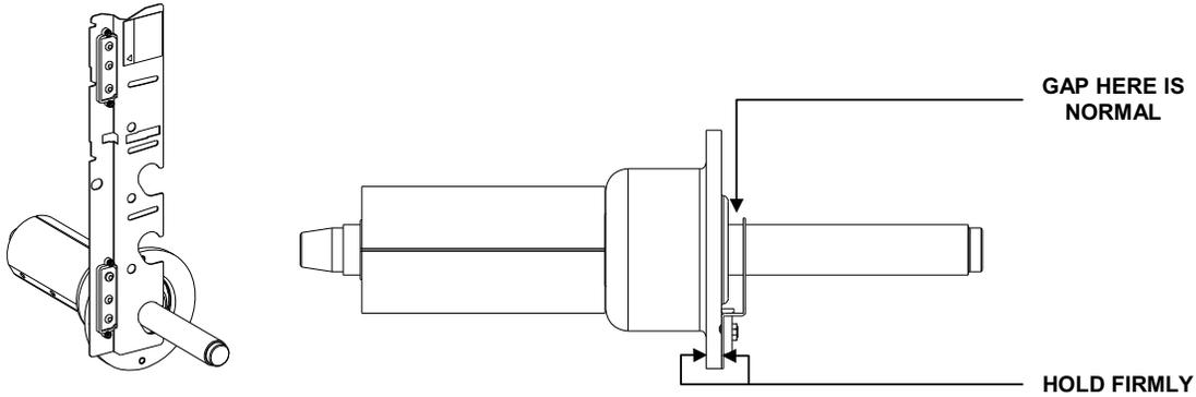
Place the outer Dataset® arm at position “1.” Tap the foot pedal once or press “Enter Cal Step.”
