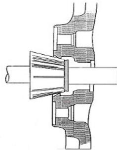
Place the wheel mounting cone on the spindle against the spring plate. Mount the wheel with the inner rim facing the balancer and centered on the cone.
