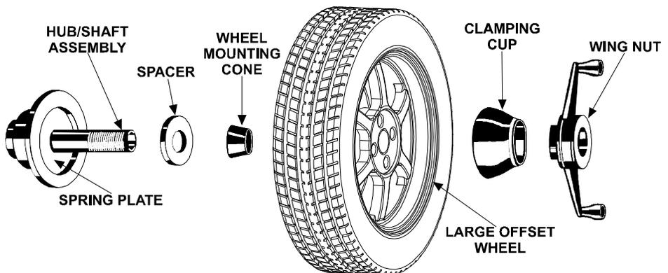
For example, one cone size is too small because the captivated spring is not pressing the cone against the inner wheel opening, but the next larger cone size is too large and will not fit the opening. Use the smaller cone size, with the spacer, to extend the captivated spring and hold the smaller mounting cone against the wheel opening with greater pressure.
