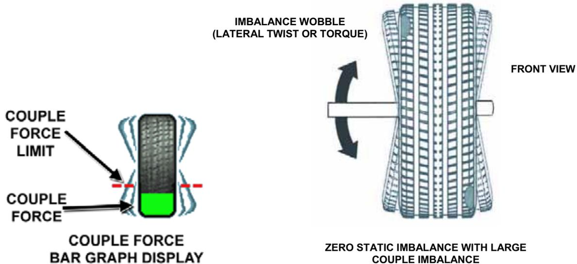
Modern “dynamic” balancers spin the wheel in order to measure both the up and down imbalance force and the wobble or shimmy related imbalance (side-to-side).
