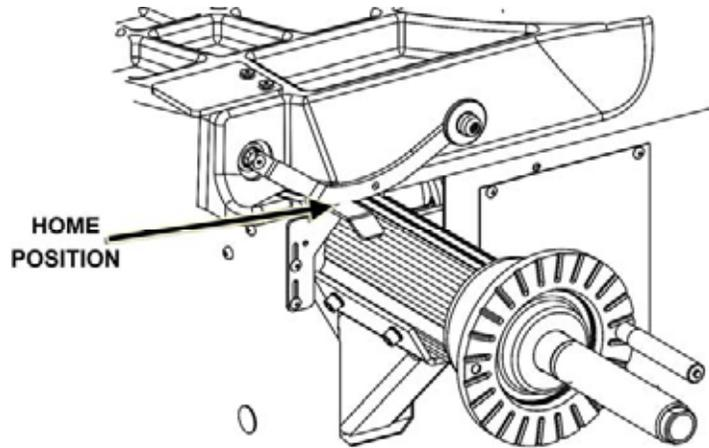
Place the calibration tool on the shaft using the middle spindle shaft slot. Align the center hole of the calibration tool with a calibration weight thread hole, and tighten the calibration weight securing the calibration tool to the hub face as shown below.
