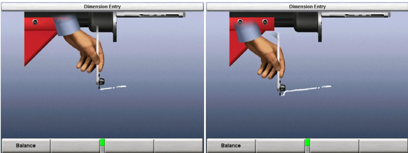
When the scan is complete, release the foot pedal and a rim illustration will appear with weight planes automatically placed at correct positions for tapers or steps.
