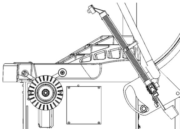
Place the calibration tool on the spindle shaft using the spindle shaft slot closest to the end of the calibration tool and hold in an upright position, flat against the hub.
