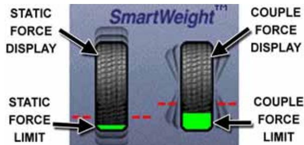
The red-dotted line represents the acceptable amount of force the tire can have that will not result in a ride problem. Any forces below that line will be shown in green. Any forces that are above that level will be shown in red and indicate an excessive amount of force.
