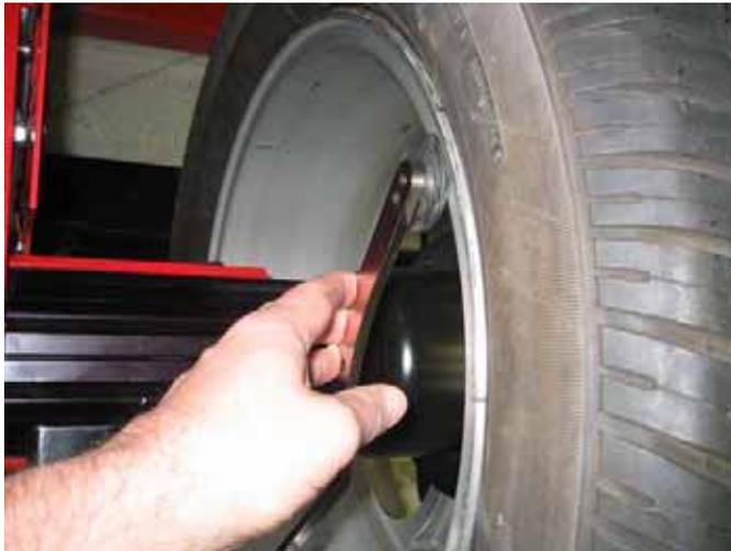
To initiate RimScan, pull the inner Dataset® arm away from the weight tray and turn to the down position.
