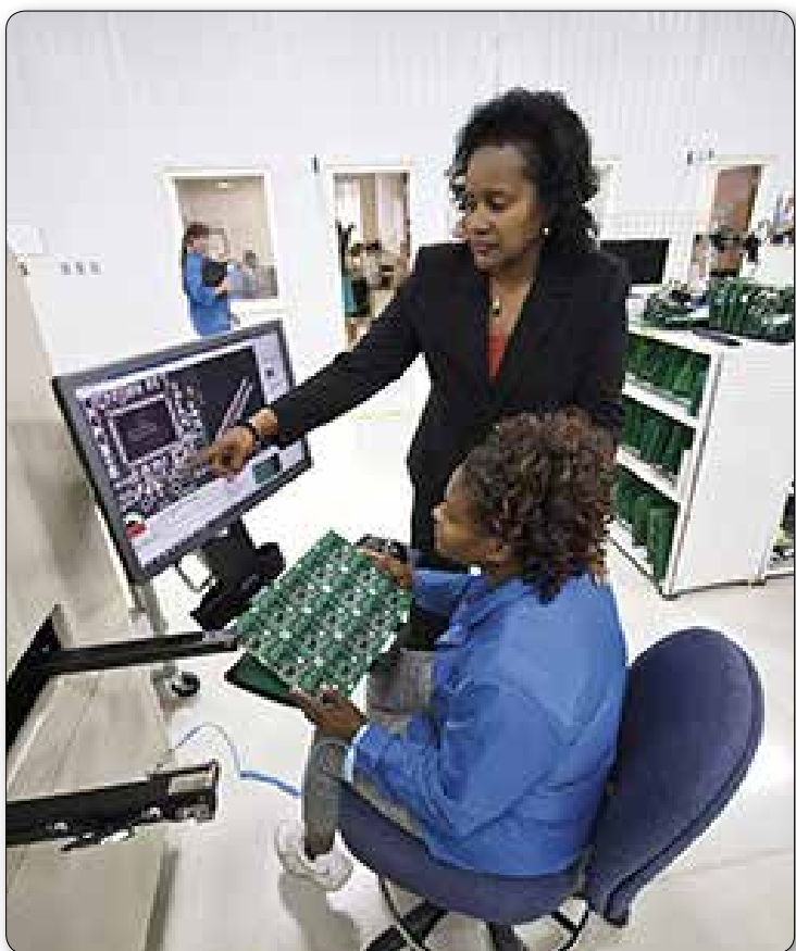
Lora oversees a wide array of quality processes including this Automated Optical Inspection (AOI) system which uses ultra-high resolution cameras to detect any misplaced components down to the micrometer level.
