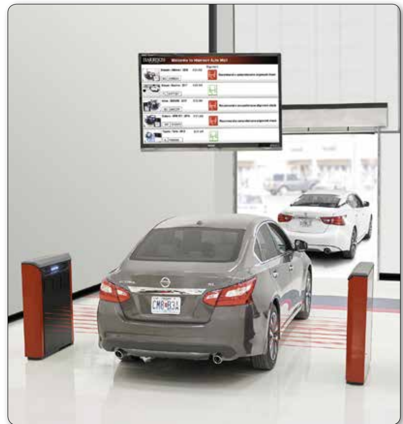
Hunter's touchless alignment inspection system uses laser technology to measure camber and total toe in seconds.
