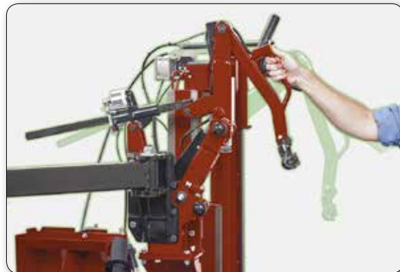
The TC37 features a traditional mount head; a polymer construction prevents damage to tire and rim.
