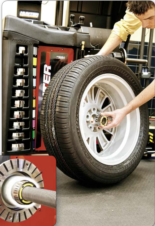
Hunter's dual taper collets provide optimized centering performance during a balancing procedure.
