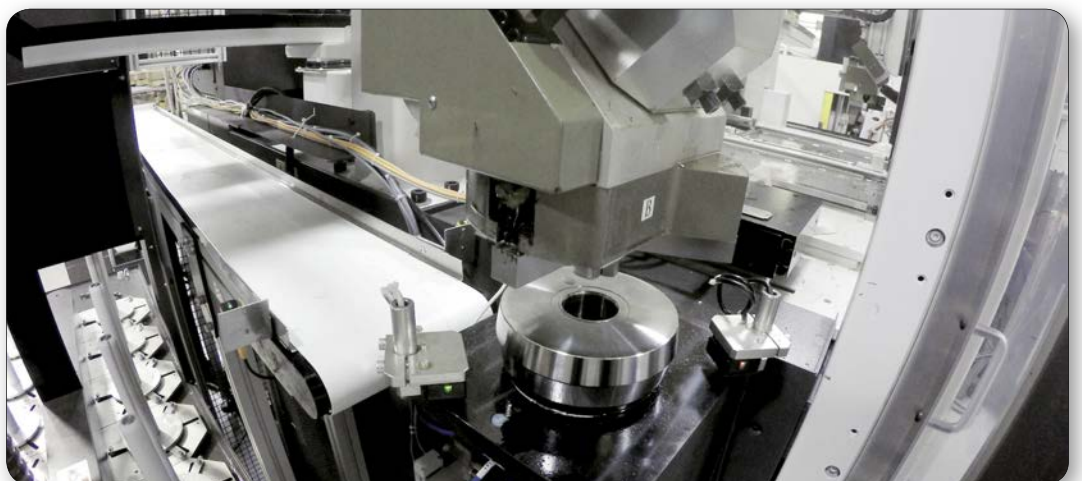
Hunter's factory produces one collet every 90 seconds with the installation of the new manufacturing cell.
